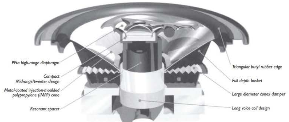
Figure 16.25 Speaker construction
