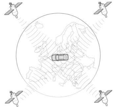
Figure 13.37 Four satellites determine vehicle position more accurately
