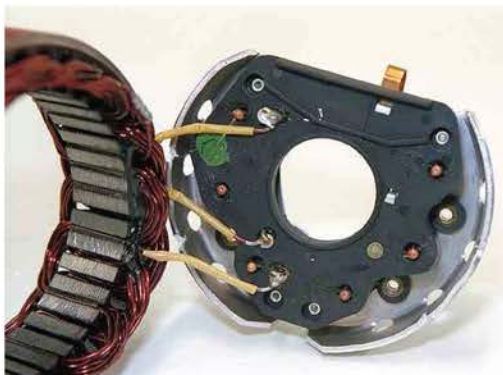
Figure 6.14 Rectifier pack and stator
