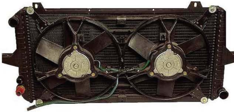
Figure 12.23 Cooling fan motor
