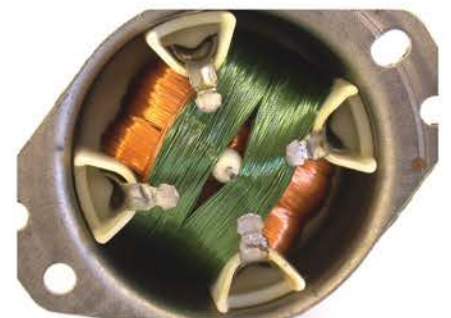
Figure 13.9 Air cored gauge unit
