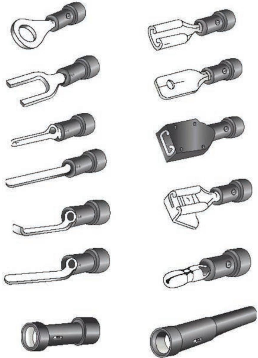
Figure 4.17 Crimp terminals for repair work
