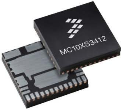
Figure 4.60 eXtreme or high side switch devices (Source: FreeScale)
