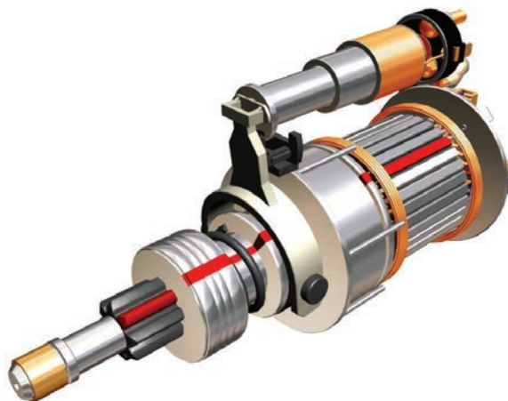
Figure 7.30 Pre-engaged starter internal components
