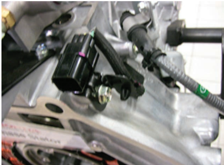
Figure 17.68 Commutation sensor connection
