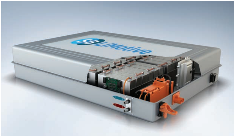
Figure 17.61 Lithium battery pack (Source: Bosch Media)
