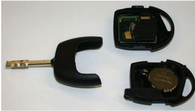
Figure 16.38 Standard key and remote transmitter combined
