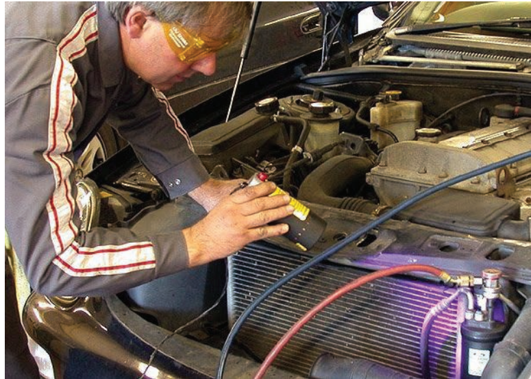
Figure 14.30 After adding a dye, leaks can be detected using a UV light
