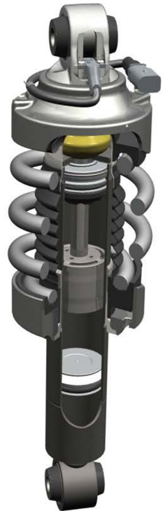
Figure 15.21 Suspension strut and actuator connection (Source: Delphi Media)
