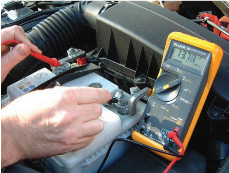
Figure 5.13 Checking battery voltage. In this case the engine had just been switched off so the reading shows a 'surface charge'
