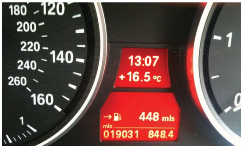
Figure 13.41 Simplified display on a BMW (MY 2009) showing time, temperature, range, mileage and trip distance
