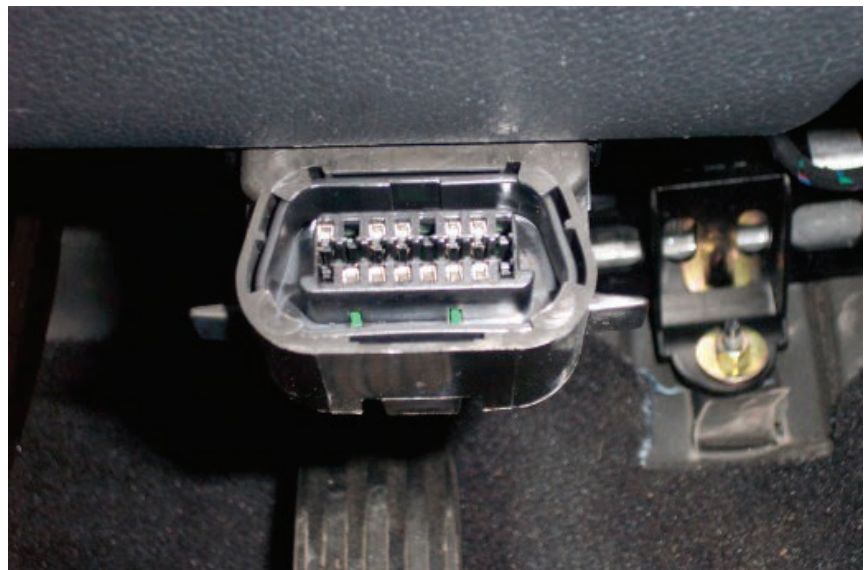
Figure 4.30 DLC socket – pin 6 is CAN-high and pin 14 is CAN-low
