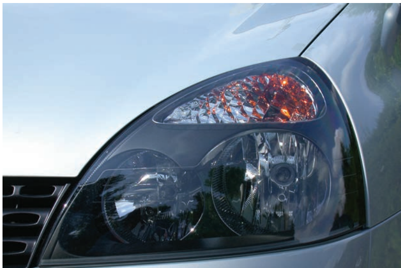
Figure 11.8 Clear lens and a complex shape reflector
