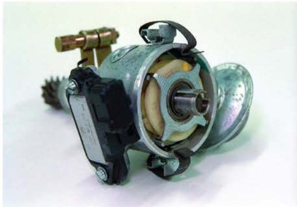
Figure 8.10 Inductive pulse generator in a distributor
