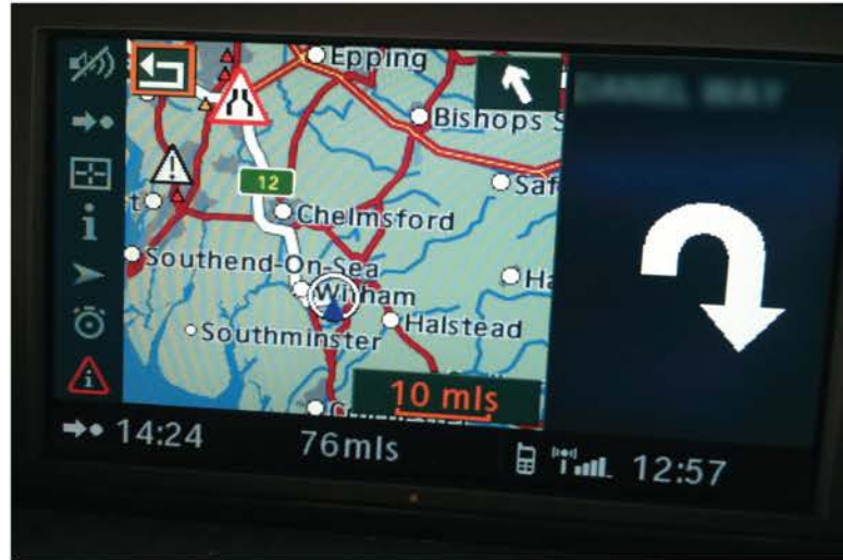
Figure 13.52 Navigation screen showing the route and additional traffic information
