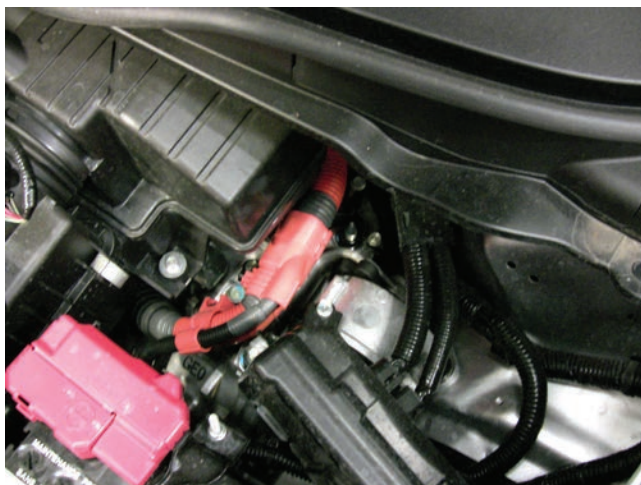
Figure 17.49 High-voltage cables are always orange
