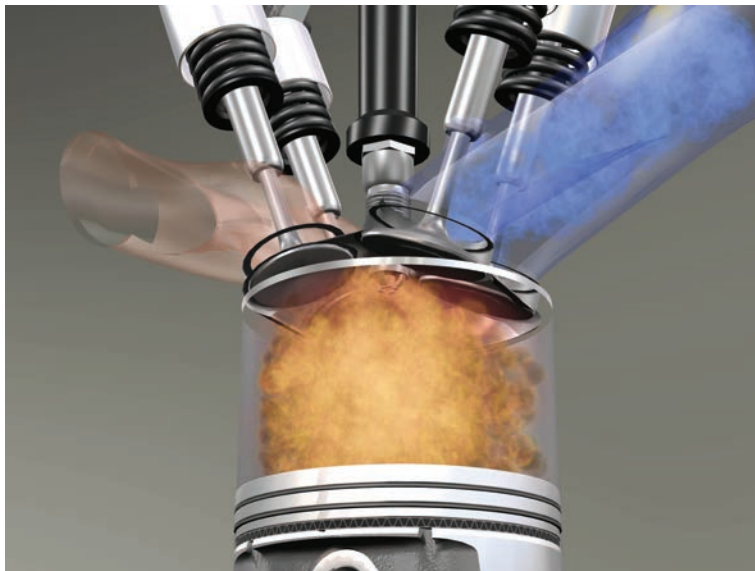
Figure 8.36 Combustion taking place (Source: Ford Media)
