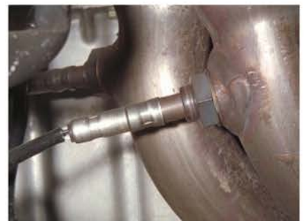
Figure 9.31 Lambda sensor in the exhaust downpipe
