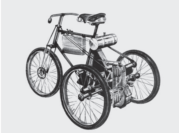
Figure 1.2 1897 The De Dion-Bouton three-wheeler, with Bosch magneto
