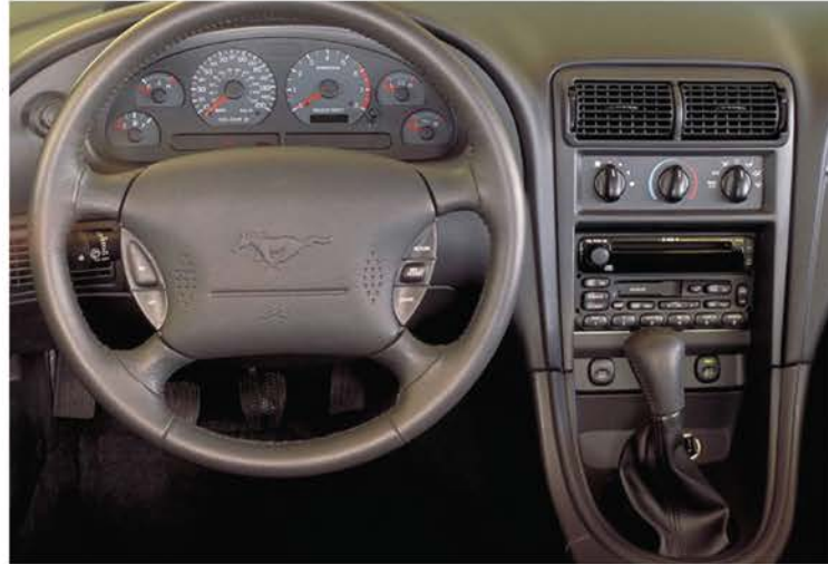
Figure 14.2 HVAC controls (top right)
