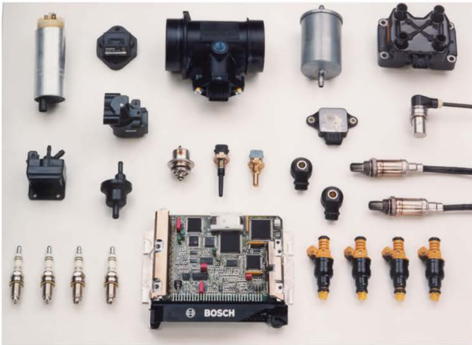
Figure 10.14 Motronic system components
