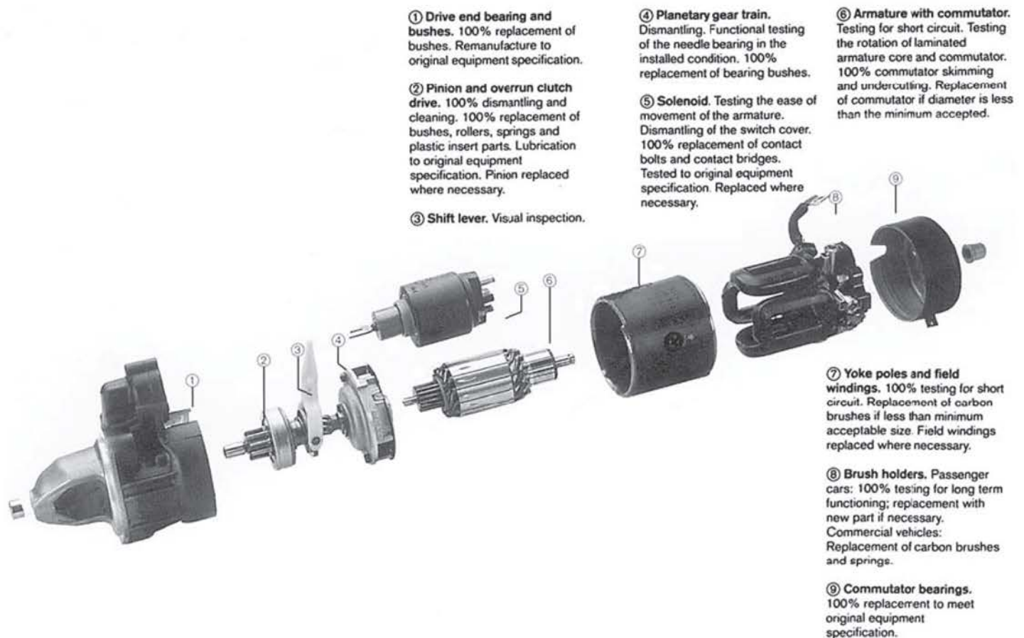
Figure 7.10 Quality starter overhaul procedure
