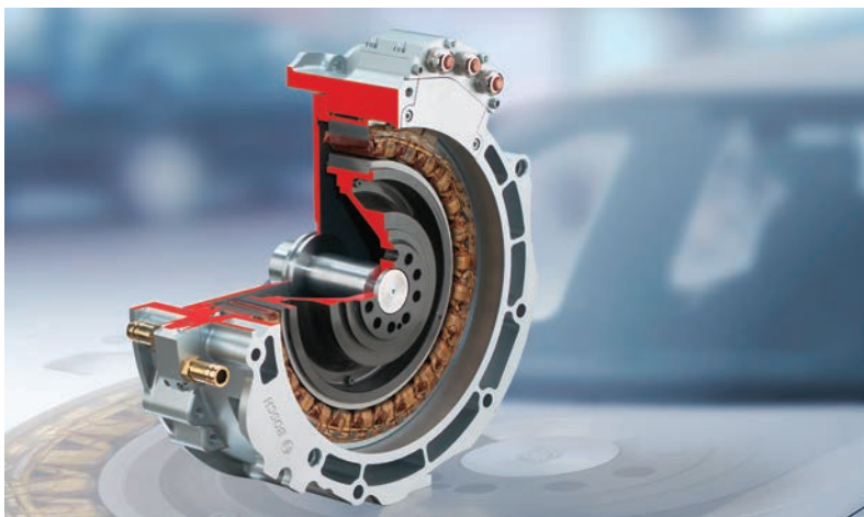
Figure 17.72 IMA motor/generator (Source: Bosch Media)
