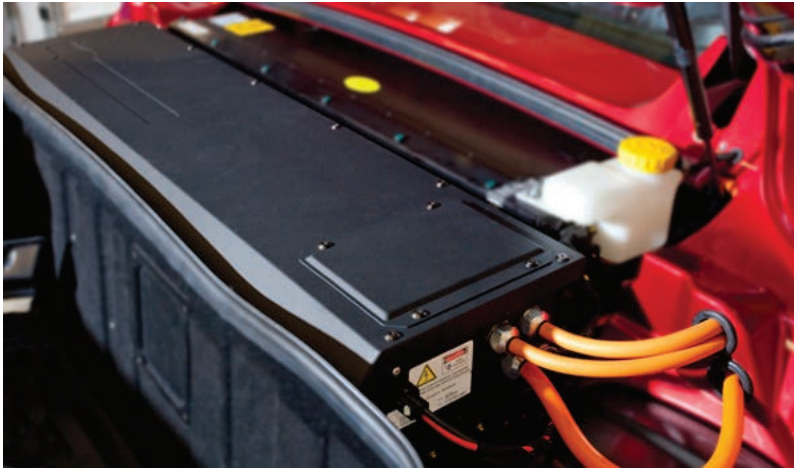
Figure 17.22 Power electronics module (Source: Tesla Motors)
