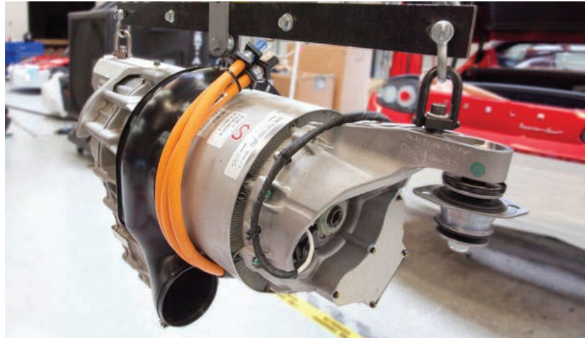
Figure 17.17 Tesla's AC induction motor (Source: Tesla Motors)
