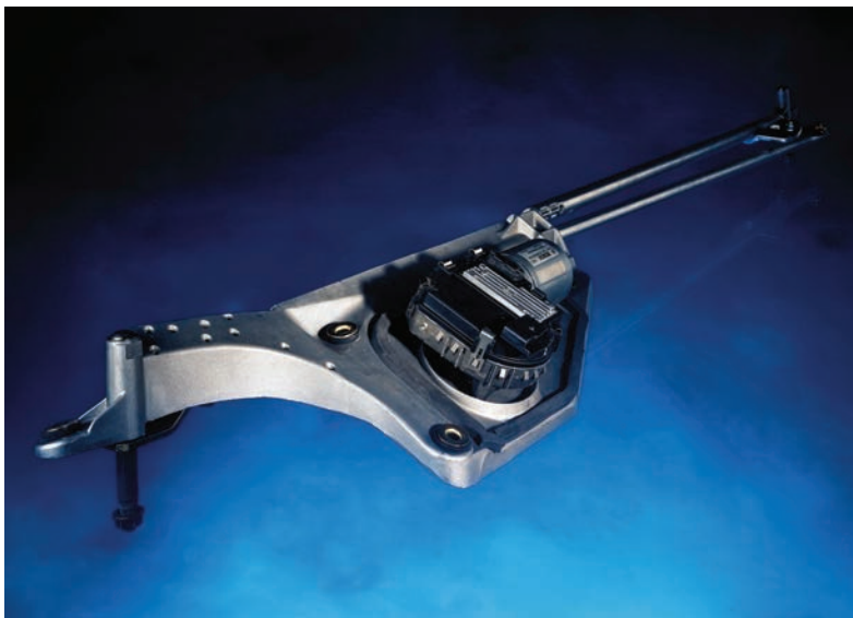
Figure 12.1 Wiper motor and linkage
