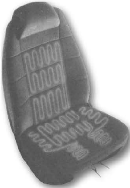
Figure 14.27 Seat containing heating element (Source: Scandmec)
