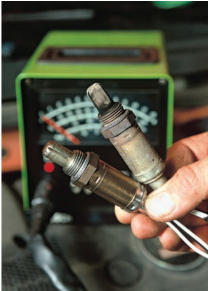
Figure 2.95 Lambda sensors performance can be tested with a voltmeter or ideally a scope
