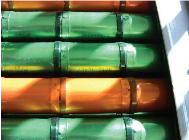
Figure 17.60 Ni-MH battery cells
