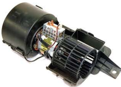
Figure 14.7 HVAC blower motor mounted in a housing
