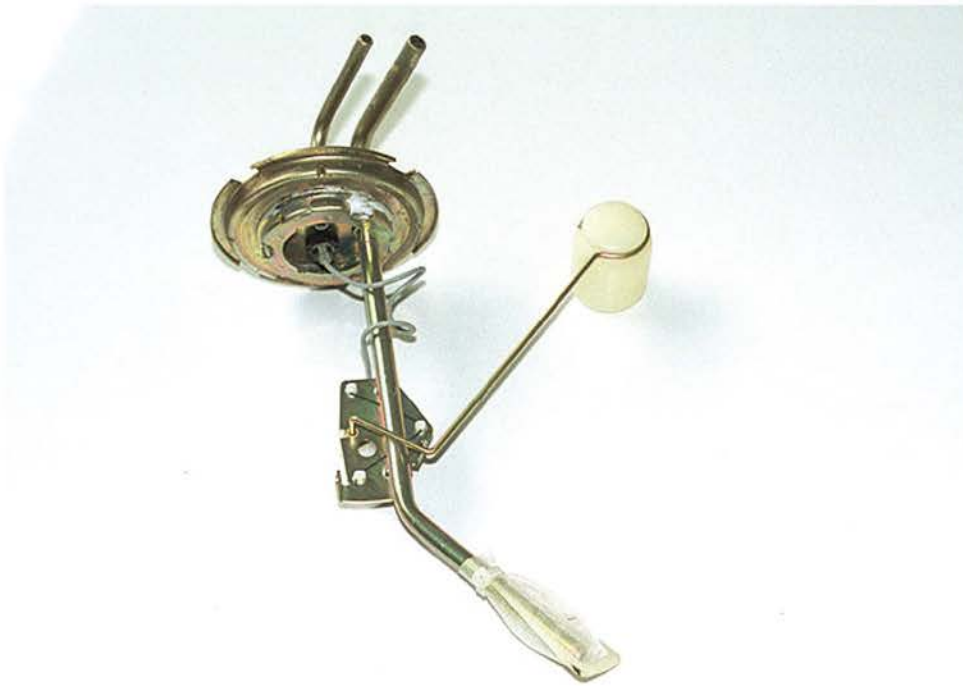
Figure 13.3 Variable resistance fuel tank unit
