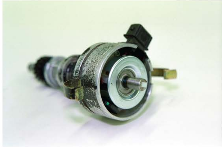
Figure 8.7 Ignition distributor with Hall generator
