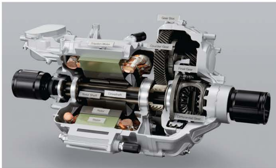
Figure 17.36 Induction drive motor, differential and final drive components (Source: Honda Media)
