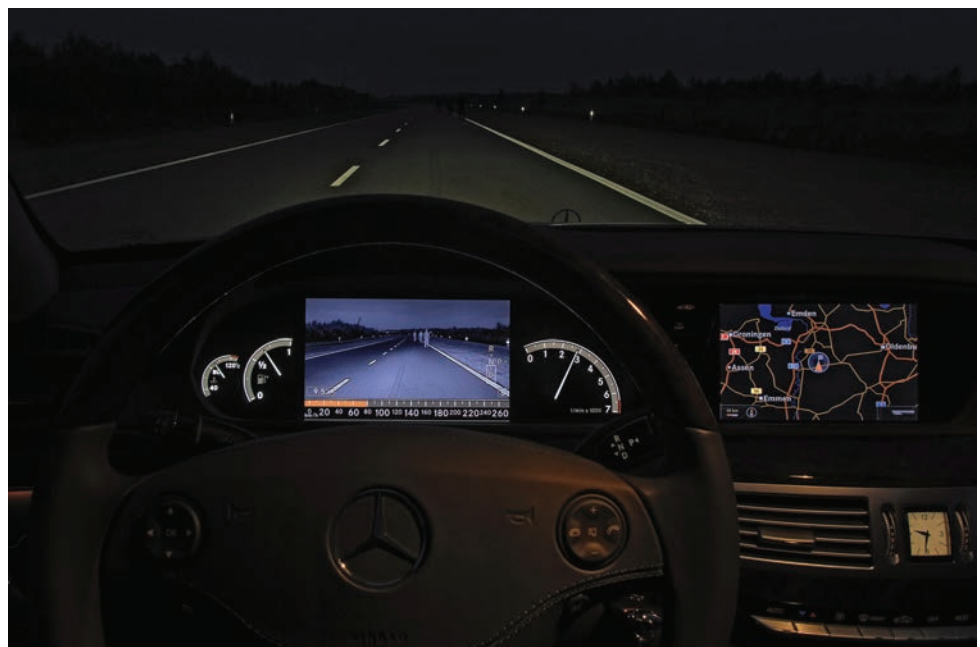
Figure 13.30 Mercedes S-Class information cluster night-vision display (Source: Bosch Media)
