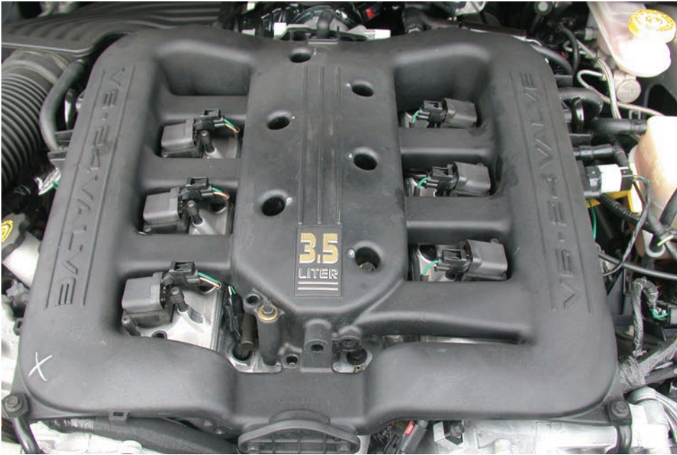
Figure 8.26 Six direct ignition coils in position
