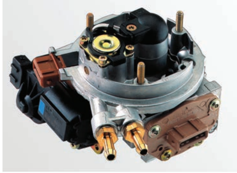
Figure 9.43 Central injection unit of the mono Jetronic
