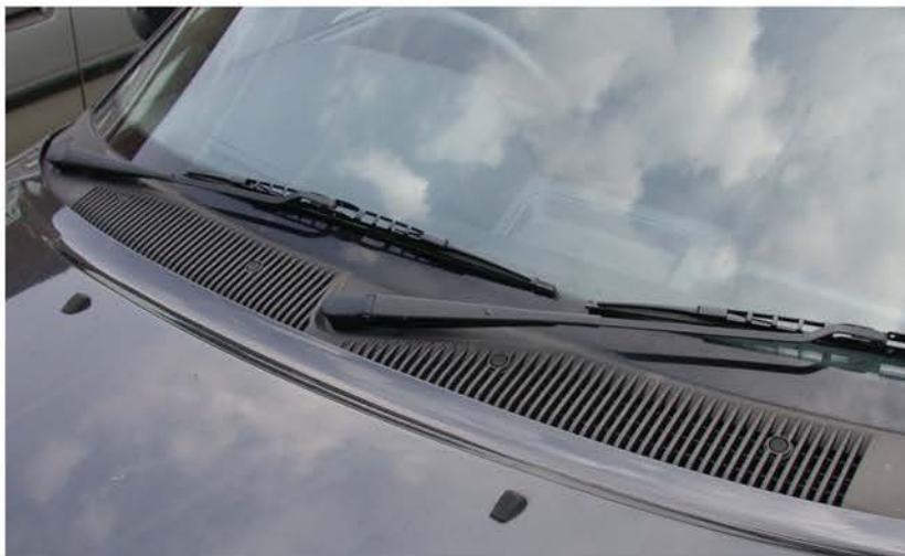
Figure 14.5 Air intake vents above the plenum chamber
