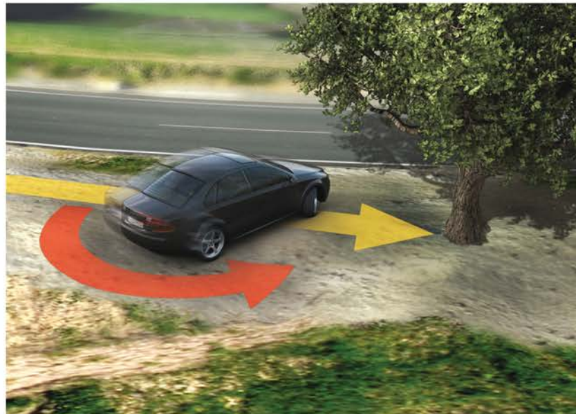
Figure 15.17 Yaw is the turning of a vehicle about a vertical axis (Source: Bosch Media)
