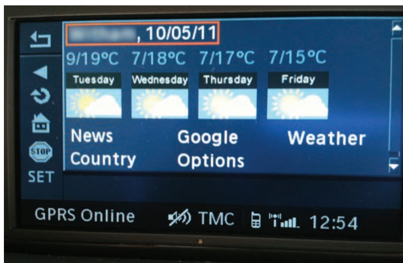
Figure 13.55 Online information relating to the vehicle's location accessed via the GPRS network
