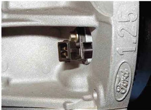
Figure 2.53 Inductive sensor on an engine
