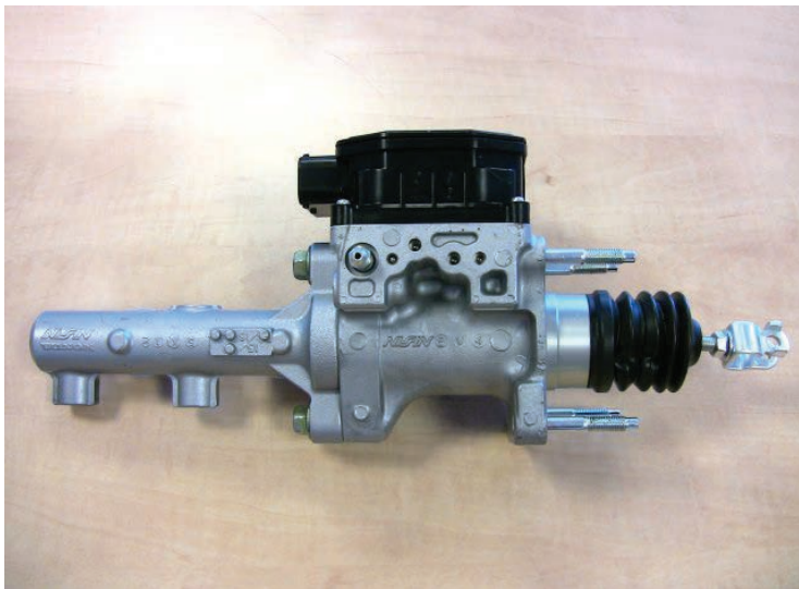
Figure 17.80 Electronically controlled brake master cylinder
