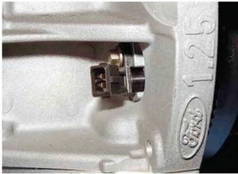
Figure 9.28 Crank sensor in position
