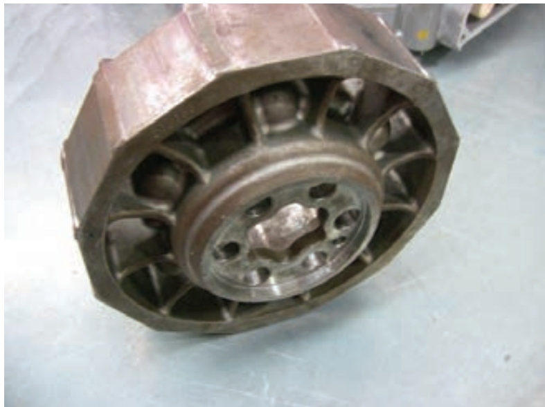
Figure 17.46 The core or rotor is made of very strong rare earth metal permanent magnets
